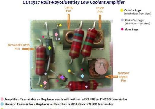
Rectifier Diode - Replace with 1N4007 or similar rectifier diode
