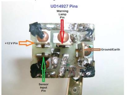
Here's what the pin arrangement on the underside of the circuit board looks like:
