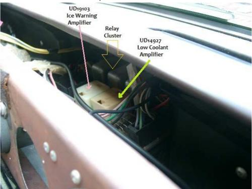
On the same board as those relays will be a whitish plastic cube, usually with its label intact, that reads: "UD 14927 Coolant Level." Carefully remove it from the relay board. After it is off the relay board, gently and carefully pry the circuit board out of the base of the cover. When that's done you should see something exactly like or very similar to this:
